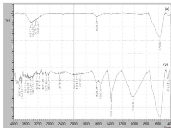
Fig. 3. The FT-IR spectra of Fe<sub>3</sub>O<sub>4</sub>-MNPs (a) before and (b) after adsorption of Cd-DTZ complex.
