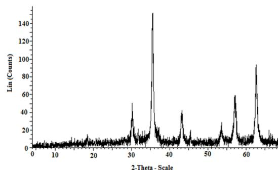
Fig. 1. XRD pattern of synthesized Fe<sub>3</sub>O<sub>4</sub>-MNPs.
