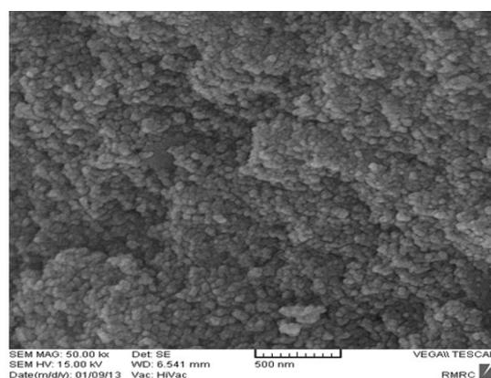
Fig. 2. SEM image of synthesized Fe<sub>3</sub>O<sub>4</sub>-MNPs.
