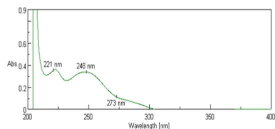
Fig. 8. Spectrum of formulation containing Carisoprodol, Paracetamol and Caffeine.
