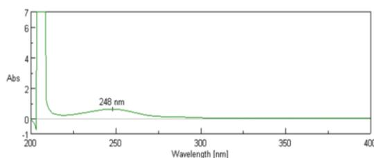
Fig. 4. UV spectra of Paracetamol
