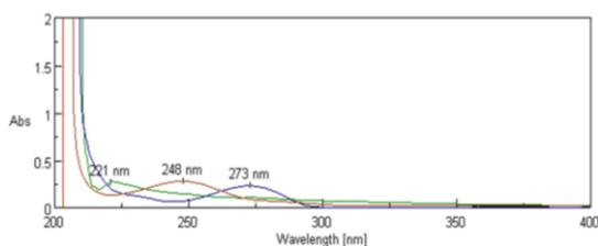
Fig.7. Overlain spectra of Carisoprodol, Paracetamol and Caffeine showing selected wavelength.
