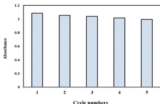
**Fig. 8.** Regeneration of Fe<sup>3</sup>O<sub>4</sub>-PDA over 5 cycles. Conditions: C DMG= 0.5 %, CNi<sup>2+</sup>= 500.0 µg/L, sorbent mass= 0.059 g, sample volume: 100.0 mL, volume of CHCl<sub>3</sub>= 1.0 mL, pH=6.6, Extraction time= 23.0 min.
