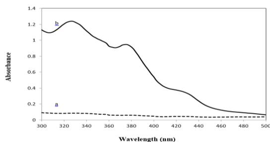
**Fig. 1.** Absorption spectra of (a) DMG and (b) its complex with Ni<sup>2+</sup> after MSPE. Conditions: C<sub>DMG</sub>= 0.5 %, C<sub>Ni<sup>2+</sup></sub>= 500.0 μg/L, sorbent mass= 0.059 g, sample volume: 100.0 mL, volume of CHCl<sub>3</sub>= 1.0 mL, pH=6.6, Extraction time= 23.0 min.
