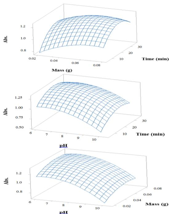
**Fig. 5.** Response surface obtained from Box–Behnken design for sorption efficiency of Ni(DMG)<sub>2</sub> complex .
