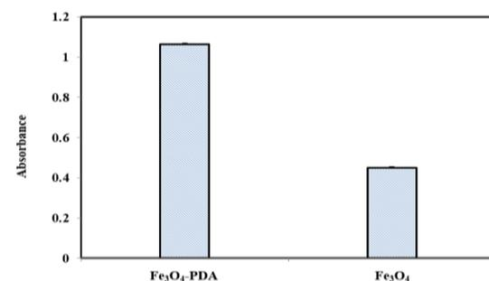
**Fig. 4.** Comparison of the extraction efficiency of Ni(DMG)<sub>2</sub> complex using Fe<sub>3</sub>O<sub>4</sub> and Fe<sub>3</sub>O<sub>4</sub>-PDA. Conditions: C<sub>DMG</sub>= 0.5 %, C<sub>Ni<sup>2+</sup></sub>= 500.0 μg/L, sorbent mass= 0.020 g, sample volume: 100.0 mL, volume of CHCl<sub>3</sub>= 1.0 mL, pH=8.0, Extraction time= 15.0 min.
