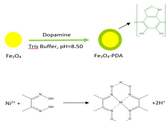
**Scheme 1.** (a) Schematic illustration for synthesis of  $\text{Fe}_3\text{O}_4$ -PDA. (b) The reaction of  $\text{Ni}^{2+}$  with DMG.
