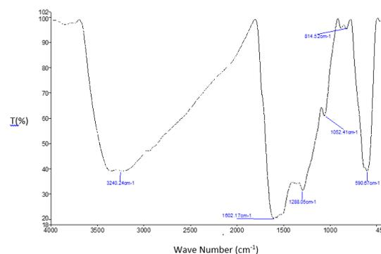
**Fig. 3.** FTIR spectrum of Fe<sub>3</sub>O<sub>4</sub>-PDA.
