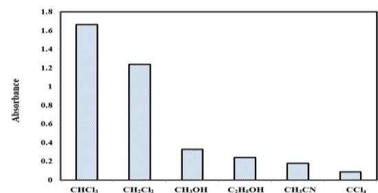
**Fig. 7.** The desorption efficiency of different eluent solvent. Conditions: C DMG= 0.5 %, C Ni<sup>2+</sup>= 500.0 μg/L, sorbent mass= 0.059 g, sample volume: 200.0 mL, desorption solvent volume = 1.0 mL, pH=6.6, Extraction time= 23.0 min.
