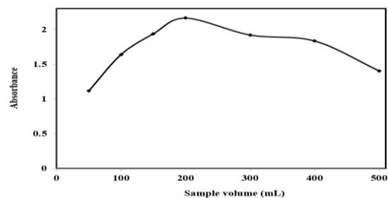
**Fig. 6.** Effect of sample volume on the sorption percentage of 500 μg/L of Ni<sup>2+</sup>. Conditions: C DMG= 0.5 %, C Ni<sup>2+</sup>= 500.0 μg/L, sorbent mass= 0.059 g, volume of CHCl<sub>3</sub>= 1.0 mL, pH=6.6, Extraction time = 23.0 min.
