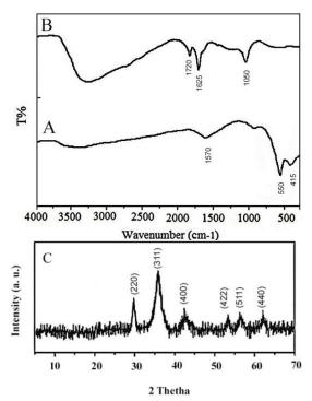
**Fig. 2.** FT-IR spectra of ZnFe<sub>2</sub>O<sub>4</sub> NPs/ reduced graphene oxide (A); pure GO (B) and XRD patterns of of ZnFe<sub>2</sub>O<sub>4</sub> NPs/ reduced graphene oxide (C).
