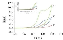
**Fig. 3.** Cyclic voltammograms of the PBS (pH 4.0) at (A) CPE ; (B) ZnFe<sub>2</sub>O<sub>4</sub>/CPE; (C) of ZnFe<sub>2</sub>O<sub>4</sub> NPs/ reduced graphene oxide /CPE and 5  $\mu$ mol L<sup>-1</sup> of bentazon in 0.1 M PBS (pH=4.0) at (D)CPE;
