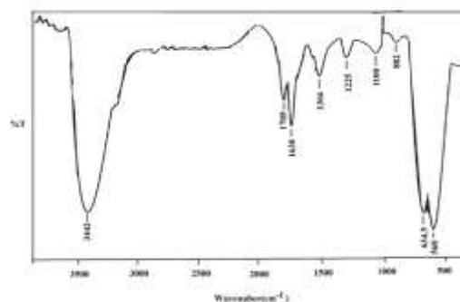
**Fig.3.** FT-IR spectrum of: Fe<sub>3</sub>O<sub>4</sub>@ $\alpha$ -Linolenic acid NPs.
