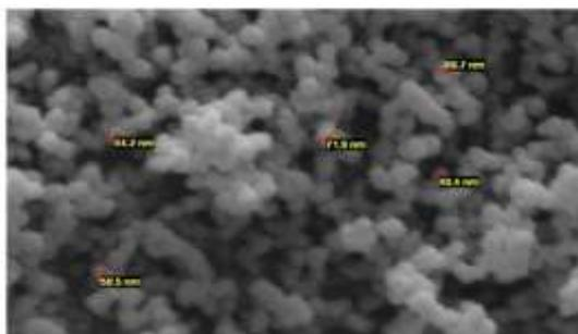
**Fig.4.** The scanning electron microscopy (SEM) of: Fe<sub>3</sub>O<sub>4</sub>@ $\alpha$ -Linolenic acidNPs.
