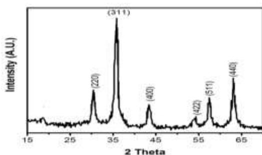
**Fig.5.** The X-ray diffraction (XRD) of: Fe<sub>3</sub>O<sub>4</sub>@ $\alpha$ -Linolenic acidNPs.
