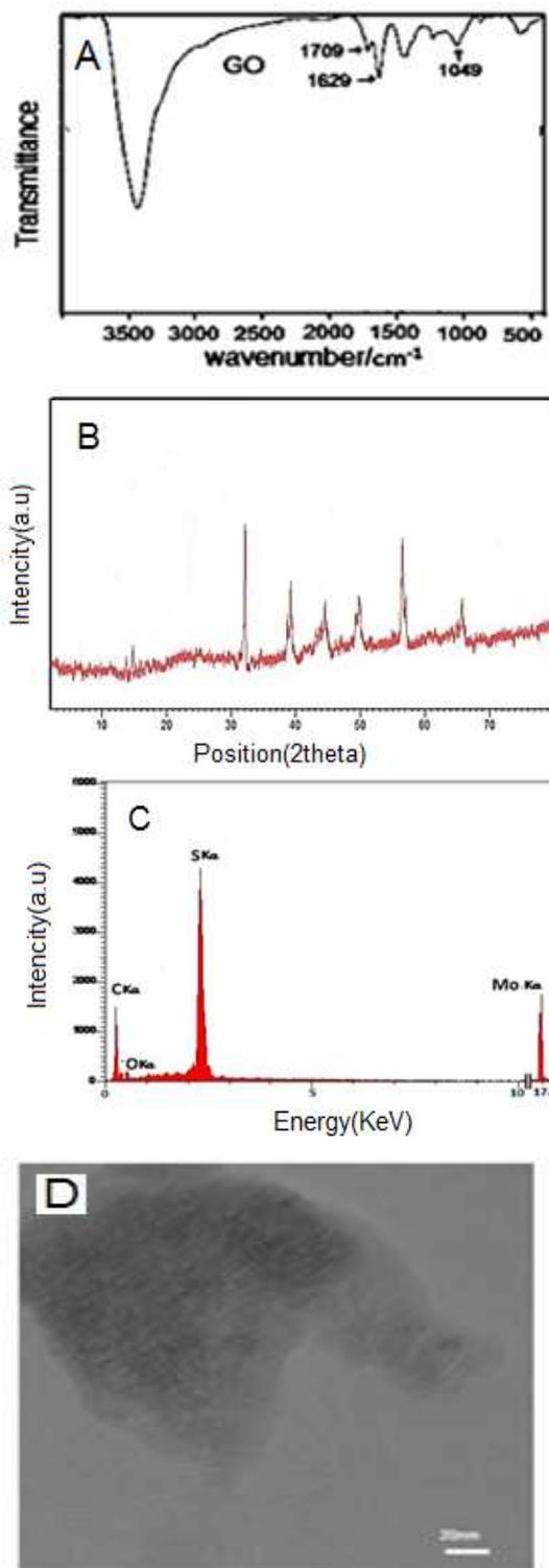
**Fig. 1.** FT-IR spectrum of synthetic graphene oxide(A), XRD pattern of the as-prepared MoS<sub>2</sub>(B), EDX elemental analysis of the as-prepared MoS<sub>2</sub>(C) and TEM image of MoS<sub>2</sub>/GO(D).
