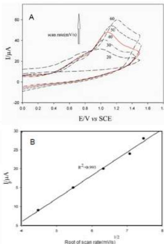
**Fig. 3.** Cyclic voltammograms of MoS<sub>2</sub>/GO-GCE inserted in 1mM of carbamazepine (pH=8) in presence of 0.1M of KCl with different potential scan rates(A), the plot of corresponded peak currents versus root of the scan rates(B).
