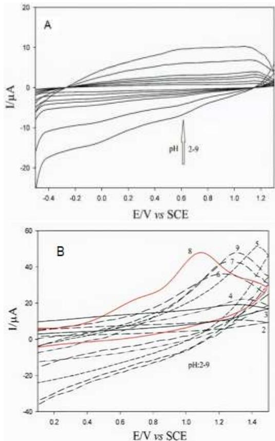
**Fig. 2.** Cyclic voltammograms of the bare GCE (A) and MoS<sub>2</sub>/GO-GCE inserted in various buffer solutions (PH=2-9) in presence of 1mM of carbamazepine and 0.1 M of KCl as the supporting electrolyte with 40 mV/s potential scan rate.
