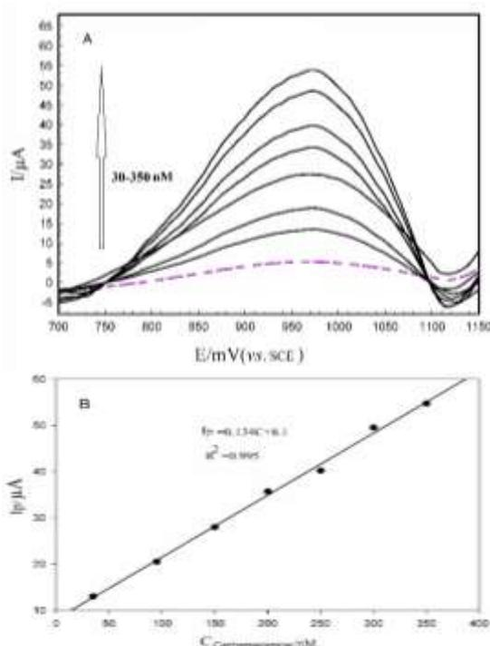
**Fig. 4.** DPV analysis of various concentrations of carbamazepine by MoS<sub>2</sub>/GO-GCE in presence of 0.1M of KCl as the supporting electrolyte (PBS, pH=8) (A) and the corresponded calibration plot(B).
