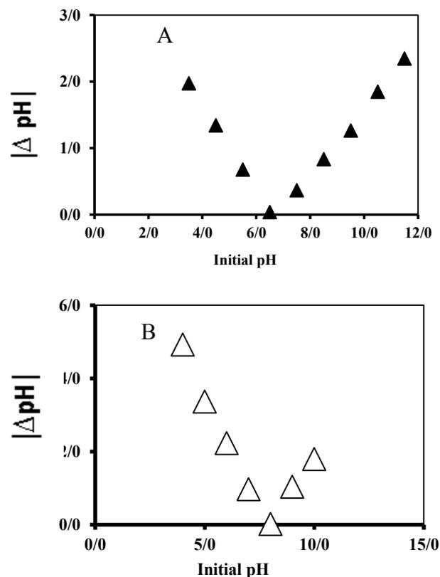
Fig. 4. Immersion technique curves of  $\text{Fe}_3\text{O}_4$ , A; and  $[\text{C}_8\text{MIM}]\text{-Fe}_3\text{O}_4$ , B.
