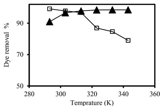
**Fig. 7.** Effect of temperature on removal of RR141 (▲) and RY 81 (□). Experimental conditions: pH 2.5, initial concentration of RR 141 (50 mg L<sup>-1</sup>) and RY81 (70 mg L<sup>-1</sup>), stirring time of 5 minutes.
