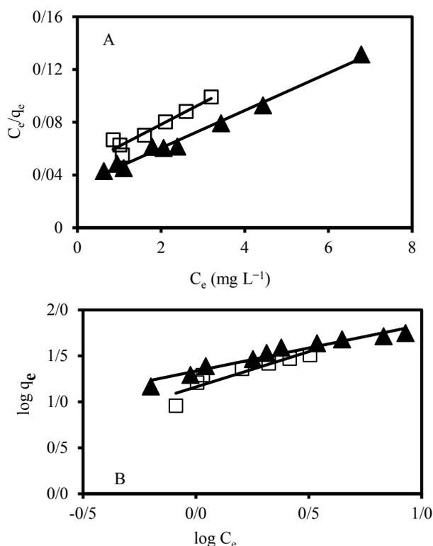
**Fig. 10.** (A), Langmuir isotherm plots; (B), Freundlich isotherm plots for adsorption of RR 141 (▲) and RY 81 (□) onto  $[\text{C}_8\text{MIM}]\text{-Fe}_3\text{O}_4$  nanoparticles. Experimental conditions:  $[\text{C}_8\text{MIM}]\text{-Fe}_3\text{O}_4$  amount of 10 mg, initial pH 2.5, stirring time of 5 minute, initial dye concentration of 50-120  $\text{mg L}^{-1}$ .
