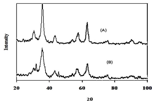
**Fig. 1.** XRD pattern of Fe<sub>3</sub>O<sub>4</sub>, A; and [C<sub>8</sub>MIM]-Fe<sub>3</sub>O<sub>4</sub>, B.
