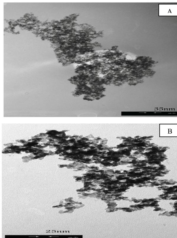
Fig. 3. The TEM image of  $\text{Fe}_3\text{O}_4$ , A; and  $[\text{C}_8\text{MIM}]\text{-Fe}_3\text{O}_4$ , B.
