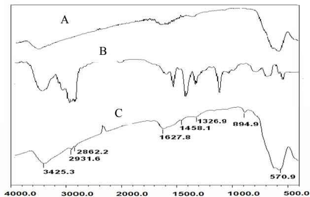
Fig. 2. FTIR spectra of  $\text{Fe}_3\text{O}_4$ , A; IL, B; and  $[\text{C}_8\text{MIM}]\text{-Fe}_3\text{O}_4$ , C.
