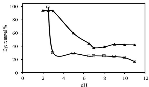
**Fig. 5.** Effect of initial pH of dye solution on removal of RR 141 (▲) and RY 81(□). Experimental conditions:  $[C_8MIM]-Fe_3O_4$  amount of 10 mg, initial concentration of RR141 (50  $mg L^{-1}$ ) and RY81 (70  $mg L^{-1}$ ), stirring time of 5 minutes.
