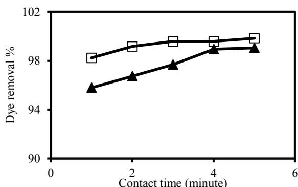
**Fig. 8.** Effect of stirring time on removal of RR141 (▲) and RY 81(□). Experimental conditions: [C<sub>8</sub>MIM]-Fe<sub>3</sub>O<sub>4</sub> amount of 10 mg, pH 2.5, initial concentration of RR 14,150 mg L<sup>-1</sup> and RY81 (70 mg L<sup>-1</sup>).
