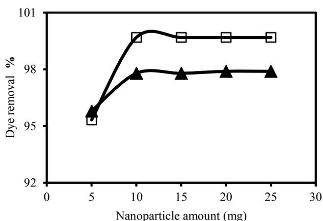
**Fig.6.** Effect of initial amount of [C<sub>8</sub>MIM]-Fe<sub>3</sub>O<sub>4</sub> nanoparticles on removal of RR141 (▲) and RY 81 (□). Experimental conditions: pH 2.5, initial concentration of RR 141(50 mg L<sup>-1</sup>) and RY81 (70 mg L<sup>-1</sup>), stirring time of 5 minutes.
