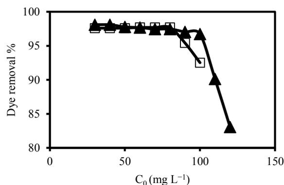
**Fig. 9.** Effect of initial dye concentration on removal of RR141 (▲) and RY 81 (□). Experimental conditions: [C<sub>8</sub>MIM]-Fe<sub>3</sub>O<sub>4</sub> amount of 10 mg, pH 2.5, initial concentration of RR 141(50 mg L<sup>-1</sup>) and RY81 (70 mg L<sup>-1</sup>), stirring time of 5 minutes.
