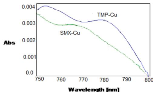
**Fig. 4.** Absorption spectra of complexes of SMX and TMP with Cu (II) in the range of 750-800 nm.
