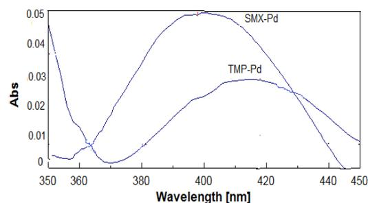
**Fig. 2.** Absorption spectra of the complexes of SMX and TMP with Pd (II) in the range of 350-450 nm.
