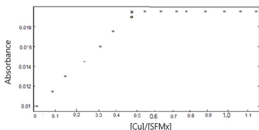
**Fig. 5.** Computer fits of the plots of absorbance vs.  $[Cu]/[SMX]$  mole ratios at 25 °C: (x) experimental point, (o) calculated point, (=) experimental and calculated points are the same within the resolution of the plots.
