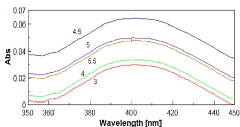
**Fig. 3.** Absorbance spectra of SMX-Pd complex in different pHs.
