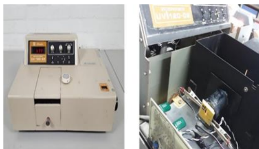
Fig. 3. (a) Shimadzu UV-120-02 Spectrophotometer (b)Replacement of the original detector with DSSC
