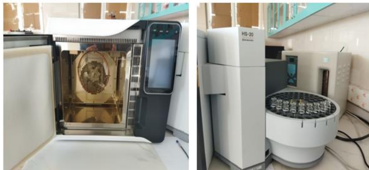
Fig. 4. The images of GC-230-FID with HS-20 headspace. A Shimadzu HS-20 headspace was used to extract the samples, and a GC-230-FID device from Shimadzu Japan was used to analyze THMs.
