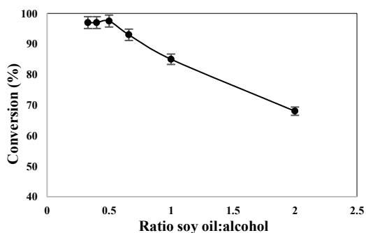
Fig. 6. Effect of oil-to- glycerol molar ratio on interesterification conversion; catalyst amount 0.5 g, reaction temperature 55 °C, molar ratio of oil to glycerol variable, reaction time 45 min.
