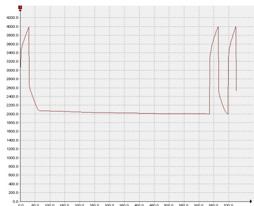
Fig. 5 b. Charge/discharge cycling curve for the Li-air battery in the presence of the LiPF 6 /DMC electrolyte and in the absence of the catalyst.
