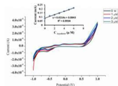
**Fig. 7.** Cyclic voltammograms of Cu/RGO-CPE electrode in 1M NaOH solution with different concentrations of the acyclovir (0-3  $\mu$ M) in scan rate 10 mV/s. The inset shows the dependency of the anodic peak current on the concentration of acyclovir in solution.
