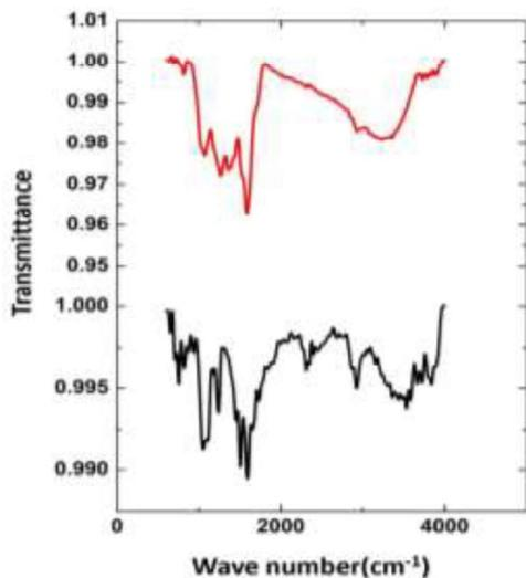
**Fig. 4.** FTIR of (a) Cu NPs and (b) Cu/ RGO
