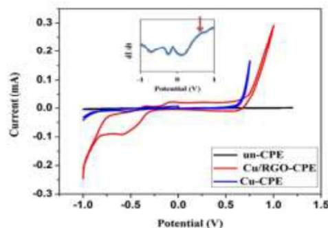
**Fig. 5.** Cyclic voltammograms of (a) un-CPE, (b) Cu - CPE and (c) Cu/ RGO- CPE in the potential range of -1-1 V in 1M NaOH. The potential sweep rate was 10 mV/s Inset: Derivative voltammogram of Cu/ RGO-CPE. The arrow indicates the location of the anodic peak.
