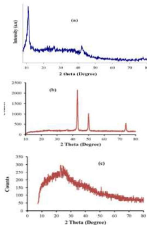
Fig. 1. XRD pattern of (a) graphene oxide, (b) Cu/ RGO and (c) Cu NPs
