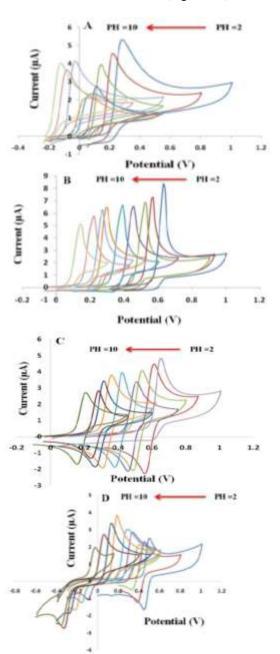
**Fig. 1.**Cyclic voltammograms of (A) AA  $(0.1\times10^{-3} \text{ mol L}^{-1})$ , (B) UA  $(0.1\times10^{-3} \text{ mol L}^{-1})$ , (C) AC  $(0.1\times10^{-3} \text{ mol L}^{-1})$ , and (D) NA  $(0.1\times10^{-3}\text{mol L}^{-1})$ , in 0.1mol L<sup>-1</sup> PBS at different pHs.
