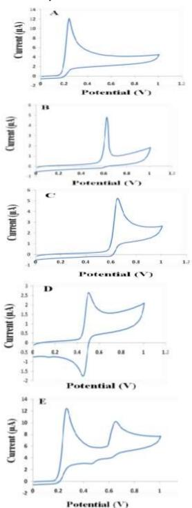
Fig. 3.Cyclic voltammograms of AA (curve a), UA (curve b), AC (curve c), NA (curve d), and their mixture (curve e) in PBS  $(0.1 \text{ mol } L^{-1}, pH \ 2.0)$ .
