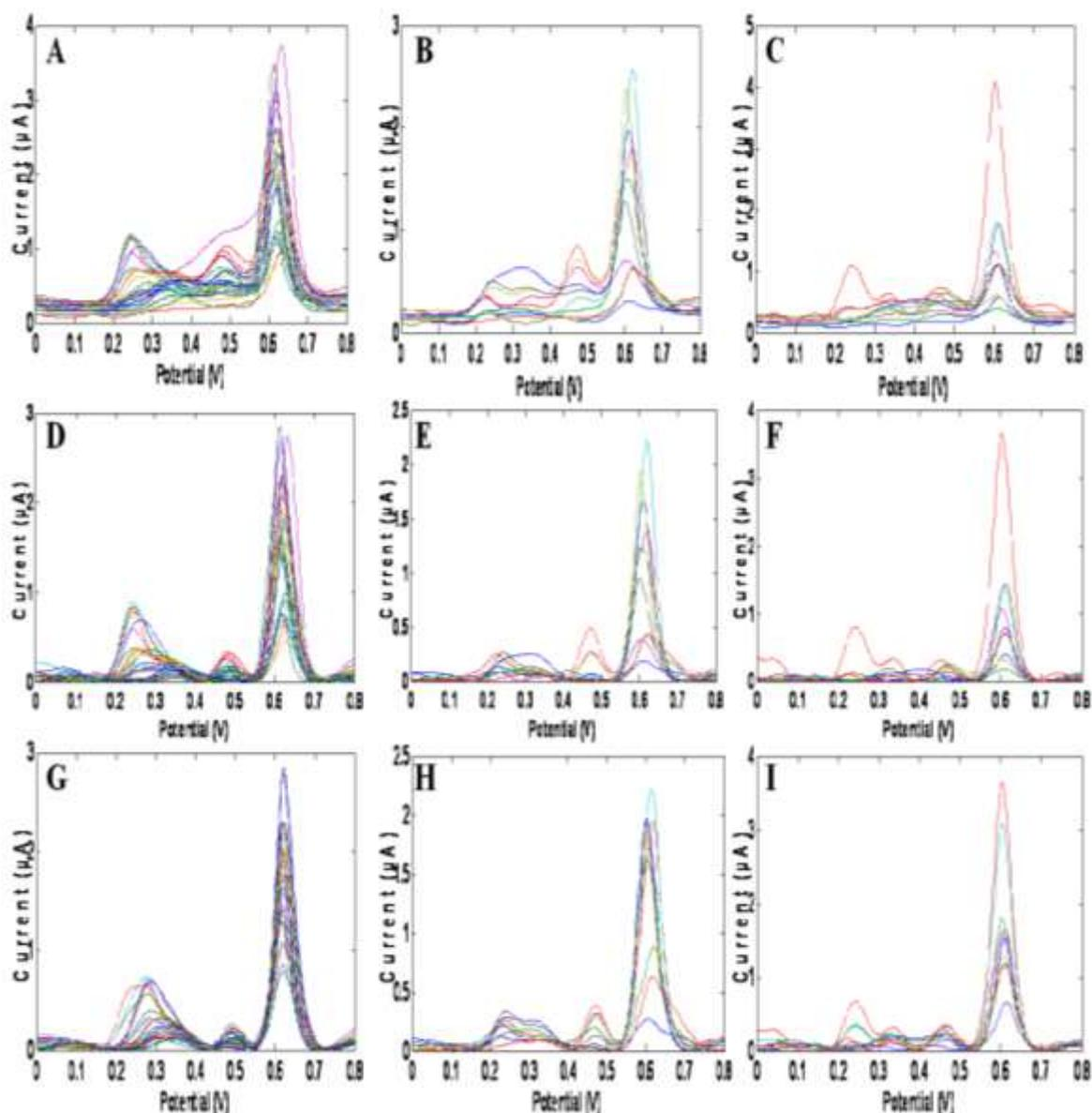
**Fig. 5.** (A)-(C): Raw data related to calibration, validation, and test sets, respectively, (D)-(F): Baseline corrected data by AsLSSR related to calibration, validation, and test sets, respectively, and (G)-(I): shift corrected data by COW related to calibration, validation, and test sets, respectively.
