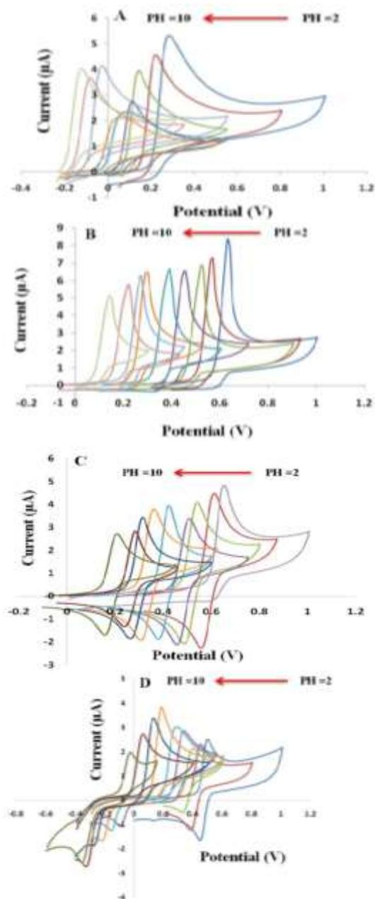
**Fig. 1.** Cyclic voltammograms of (A) AA ( $0.1 \times 10^{-3} \text{ mol L}^{-1}$ ), (B) UA ( $0.1 \times 10^{-3} \text{ mol L}^{-1}$ ), (C) AC ( $0.1 \times 10^{-3} \text{ mol L}^{-1}$ ), and (D) NA ( $0.1 \times 10^{-3} \text{ mol L}^{-1}$ ), in  $0.1 \text{ mol L}^{-1}$  PBS at different pHs.
