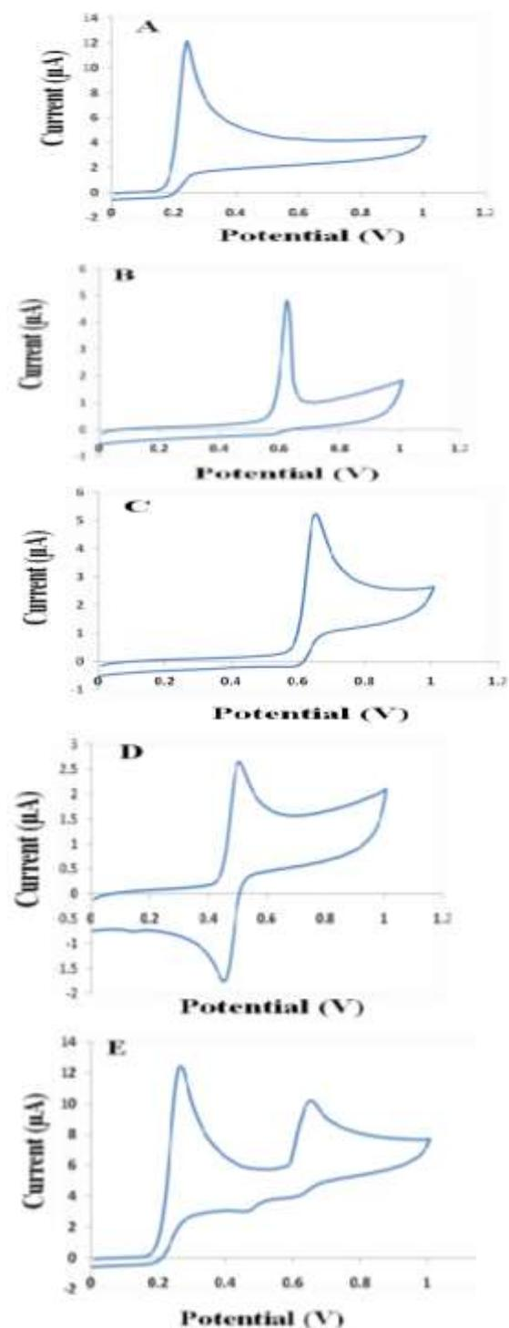
**Fig. 3.** Cyclic voltammograms of AA (curve a), UA (curve b), AC (curve c), NA (curve d), and their mixture (curve e) in PBS (0.1 mol L<sup>-1</sup>, pH 2.0).
