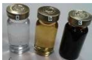
Fig. 2. Digital optical images of (a), \text{AgNO}_3 (10 mM), (b) leaf beet sugar extracted and (c) nanosilver solution
