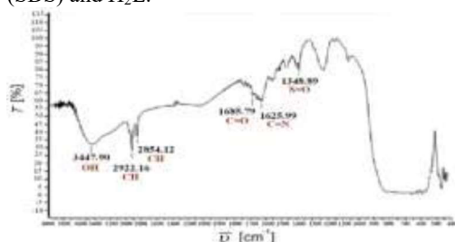
Fig 1. The FTIR spectra of H 2 L-SDS-A The SEM and TEM image of adsorbent shown in
