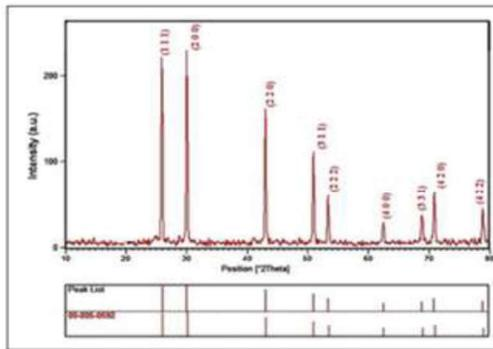
**Fig. 4:** The (a) FT-IR transmittance spectrum image and (b) XRD of the preparation of synthesized PbS Quantum Dot-Gelatin Nano composites.
