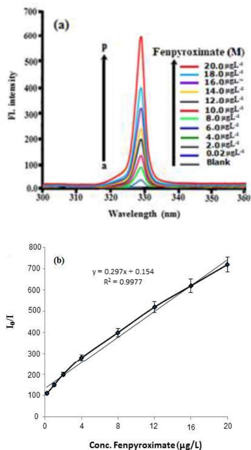
**Fig.7.** (a) Fluorescence emission intensity for determination toxic fenpyroximate by PbS Quantum Dots–Gelatin nanocomposite in width gap is 5 nm from (0.02 to 20.0  $\mu\text{g L}^{-1}$ ) of toxic fenpyroximate (b) toxic fenpyroximate Calibration curve diagram (0.02–20.0  $\mu\text{g L}^{-1}$ ) solution,  $2.5 \times 10^{-3}$  M of PbS Quantum Dot–Gelatin nanocomposites, pH 6.0, time 40 s, in phosphate buffer.
