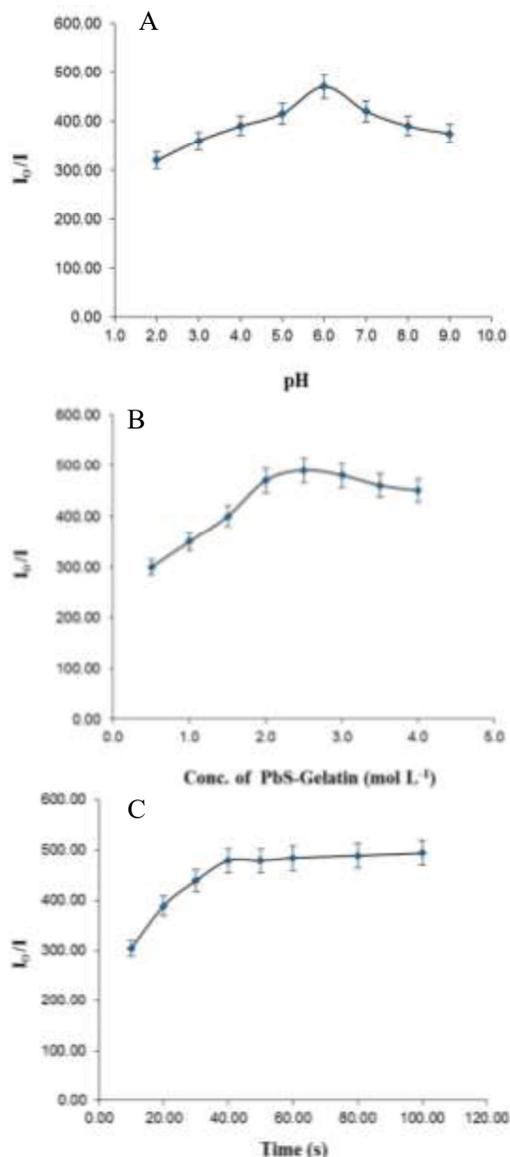
**Fig.6.** A) The impact of pH in the fluorescence intensity rate, PbS Quantum Dot–Gelatin nanocomposites,  $2.5 \times 10^{-3}$  M, glutaraldehyde (25%), time 40 s, 328 nm). B) The impact of PbS Quantum Dot–Gelatin nanocomposites in the fluorescence intensity rate. glutaraldehyde (25%), pH 6, time 40 s, 328 nm). C) The impact of time in the fluorescence intensity rate. PbS Quantum Dot–Gelatin nanocomposites,  $2.5 \times 10^{-3}$  M, glutaraldehyde (25%), pH 6, 328 nm).
