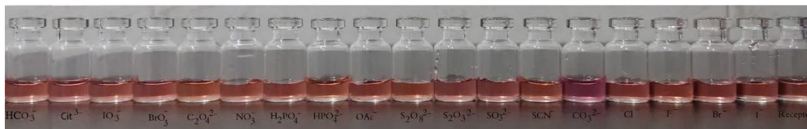
Fig. 1. Naked-eye visible color changes of UV-Vis spectra of ALRS/CR (60:40 v/v, ALRs and CR solution. 50 \mu\text{mol L}^{-1} ) in DMSO/H 2 O (25:75 v/v, HEPES buffer solution 10 \text{ mmol L}^{-1} , pH=8.5) in the presence of 1.25 \times 10^{-3} \text{ mol L}^{-1} of different anions (I - , Br - , F - , Cl - , SCN - , SO 3 2- , S 2 O 3 2- , S 2 O 8 2- , OAc - , HCO 3 - , H 2 PO 4 - , HPO 4 2- , NO 3 - , C 2 O 4 2- , Cit 3- , Bromate and IO 3 - ions) and 1.07 \times 10^{-4} \text{ mol L}^{-1} carbonate ions.
