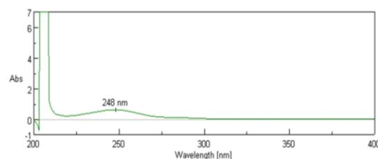
Fig. 4. UV spectra of Paracetamol
